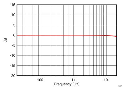
Figure 15. Soundbar Frequency Response
