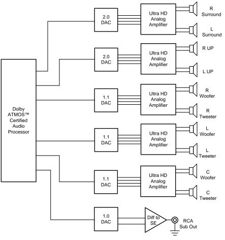
Figure 1. TIDA-01414 Block Diagram
