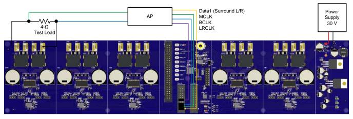
Figure 14. Soundbar Test Setup
