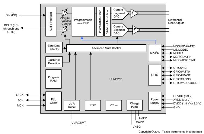
Figure 3. PCM5252 Block Diagram
