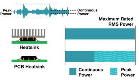
Figure 8 shows the benefits of a space-saving pad-down design for the TPA3244 amplifier.
