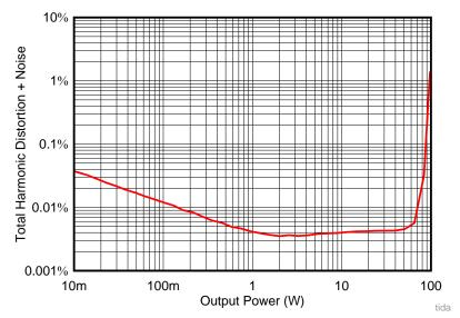
Figure 17. Total Harmonic Distortion + Noise versus Power
