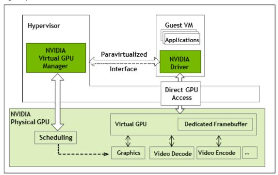
NVIDIA GRID software installed on a hypervisor manages the scheduling of GPU resources among various VMs. Each VM has its own dedicated frame buffers based on allocation. The GPU and the video encoder and decoder are shared resources that are controlled by the scheduling policy.
