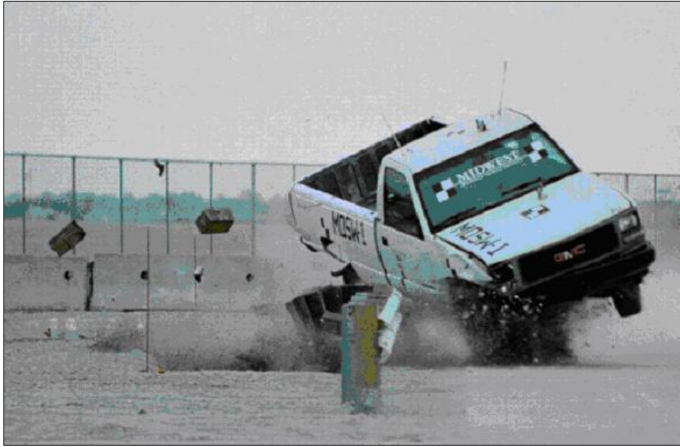
Figure 4. A pickup truck strikes a W-beam guardrail in a full-scale crash test
