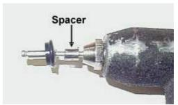
Next, the rubber buffers are installed using the 3/16 inch rivets and stainless flat washers.
