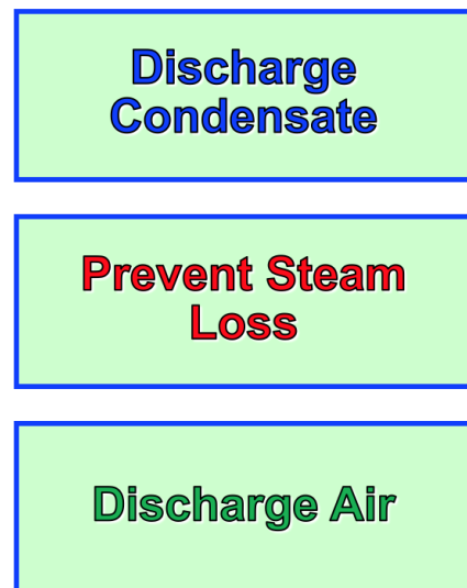
▲ Figure 7. A steam trap has 3 functions, but this article deals mostly with the first two.
