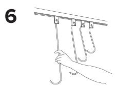
Insert the hooks through the holes in the tabs that are hanging down from the Trolleys. Each hook length should be at least 3" different than the neighboring hook.
