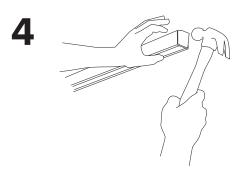
Hammer an End Cap into one end of the 96" Slotted Track.
