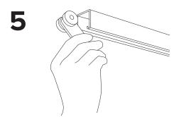
Insert the Trolleys into the open end of the 96" Slotted Track.
