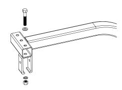
Fasten the Channel Supports to the uprights with ½" x 3" bolts, ½" washers, ½" lock washers, and ½" nuts.
