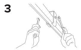
Secure the Channel Trolley Supports onto the 96" Slotted Track by tightening the Hex Head Cap Screws and Flange Nuts through the holes in the Channel Trolley Supports.
