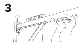
Make sure the horizontal Slotted Track is level. Adjust if necessary.
