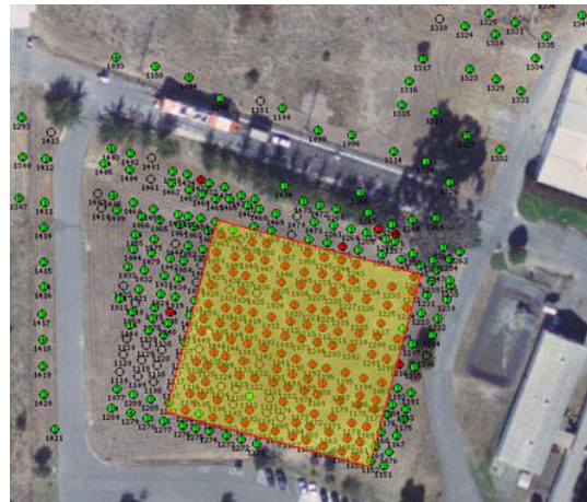
Fig. 14. Sensor network deployment (not all deployed sensor nodes are shown). The disks and circles represent the positions of the sensor nodes. The network of 144 nodes used in the multi-target tracking and PEG experiments is highlighted.
