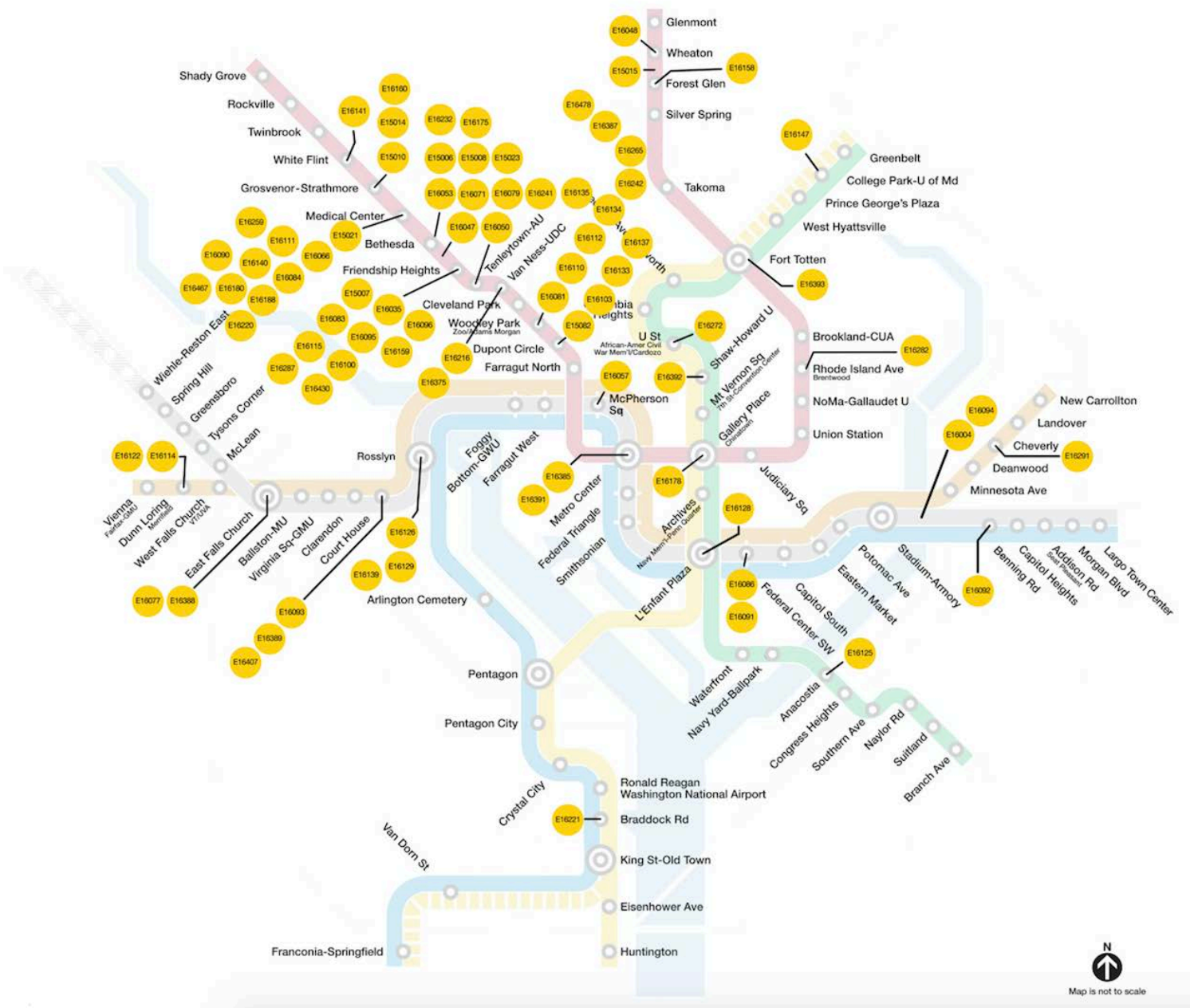
Figure 1: Electrical Arcing Events with Smoke/Fire between October 26, 2015 and October 21, 2016
