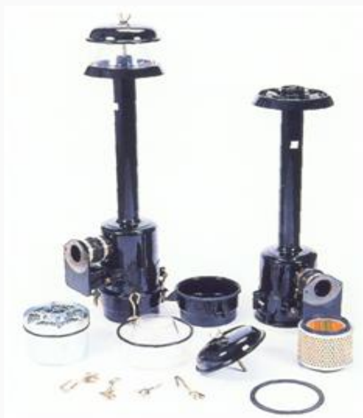
Fig. 5.3: Oil bath type air cleaner assembly
