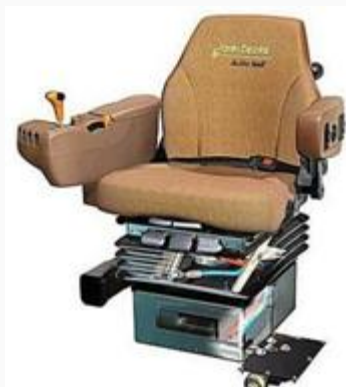
Fig. 13.2 Modern seat using “active seat” technology (CourtesyJonhDeere, 2013)
