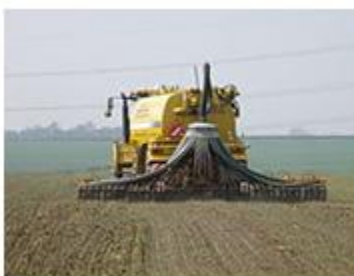
Fig 12.8: Agricultural slurry applicator using crab steering to minimise soil compaction
