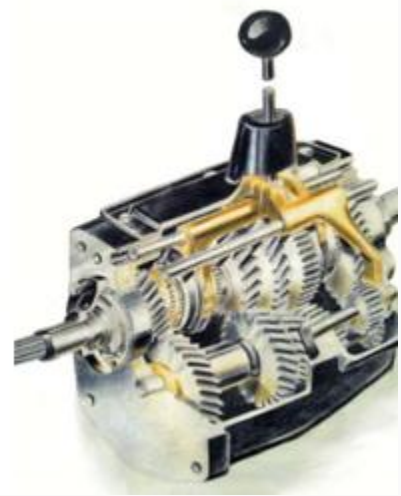
Fig. 11.7: Simple unsynchronized systems (Source: http://wikicars.org/images/en/thumb/c/c8/Gearbox_diagram.JPG/400px-Gearbox_diagram.JPG )
