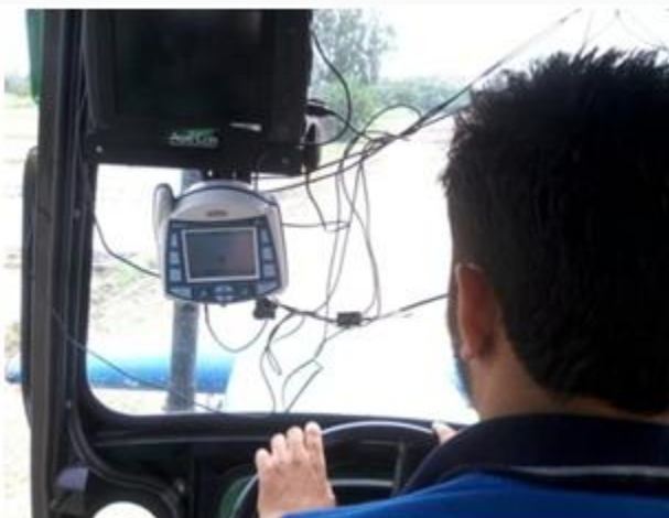
Fig. 20.2: Tractor with satellite navigator (ARAG, Italy)
