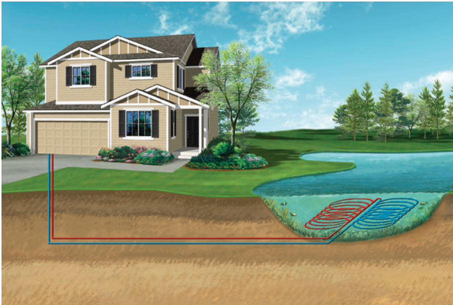
Fig. 12 Lake/pond closed loop geothermal cooling system
