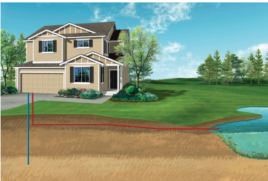
Fig. 13 Lake/pond open loop geothermal cooling system
