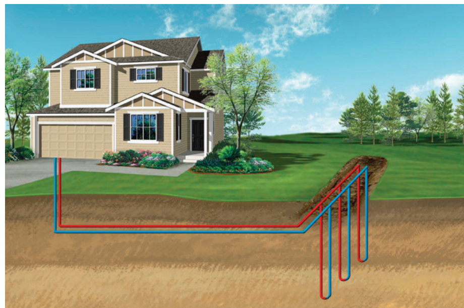
Fig. 11 Vertical closed loop geothermal cooling system
