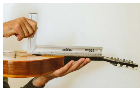
Picture 0.2 Inspection of the instrument with a ruler – view from the ending and side-view
