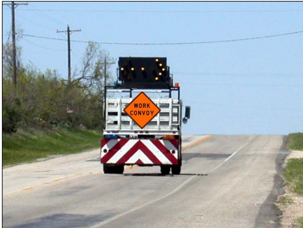
Figure 20. Current Setup Used on Two-Lane, Two-Way Roadways with Improved Shoulders.
