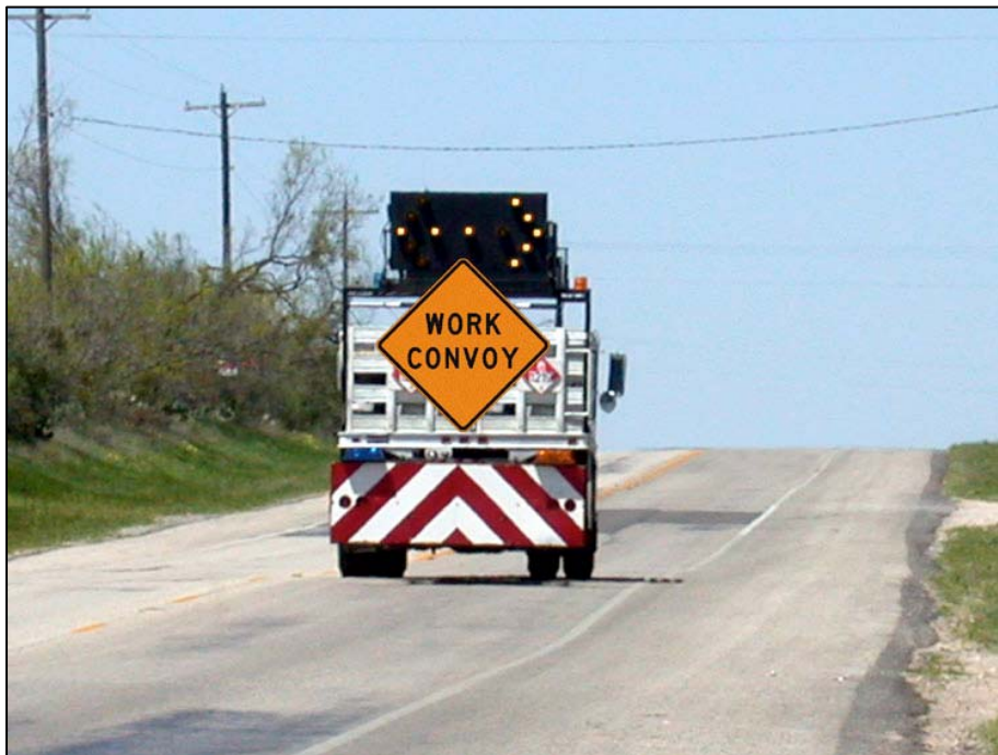
Figure 7. WORK CONVOY Sign and Four-Corner Caution Arrow Panel Display on Work Vehicle (TLTW Roadway with Improved Shoulders).
