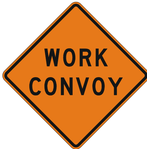
Figure 3. WORK CONVOY Sign (CW21-10).
