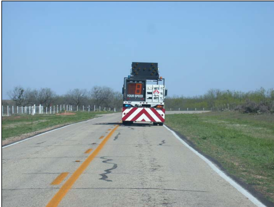
Figure 1. Mobile Speed Display Used by the San Angelo District.
