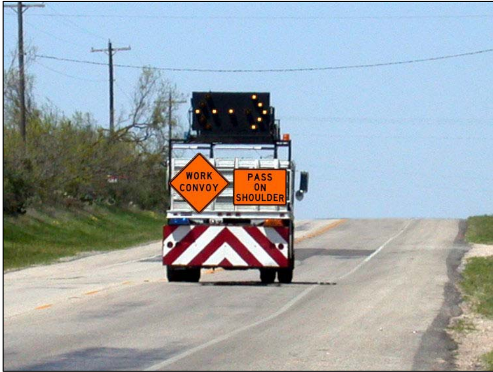
Figure 21. Addition of a PASS ON SHOULDER Sign.
