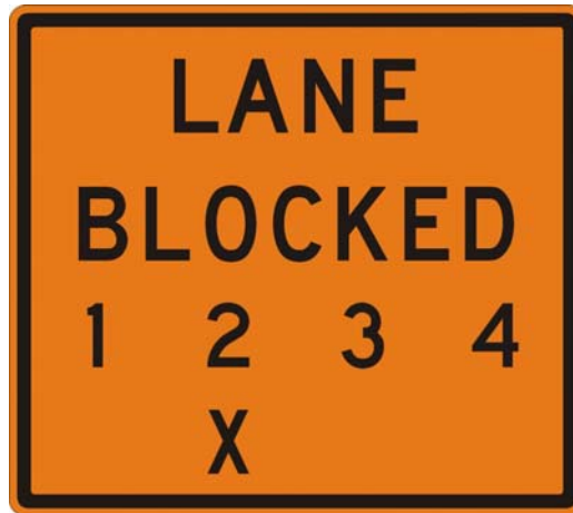
Figure 10. LANE BLOCKED Sign (FCW20-6).
