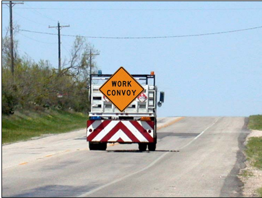
Figure 6. WORK CONVOY Sign on Work Vehicle (TLTW Roadway with Improved Shoulders).
