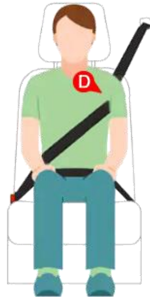
Incorrectly Fitted Seat Belts
