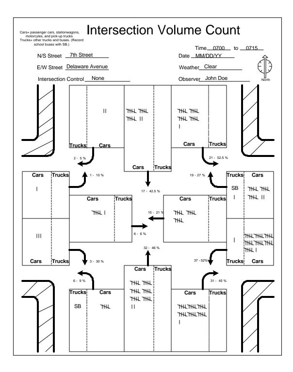
Figure 3.4. Example Manual Intersection Volume Count Tally Sheet
