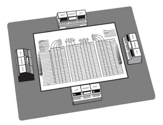
Figure 3.1. Mechanical Counting Board
