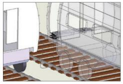
Figure 1-4 – Turn transfer bridge  $90^\circ$  and carefully unfold top section (one fold) as shown.
