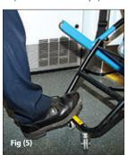
Align EVAC-CHAIR with top of folding stair and use foot to retract inner wheels.
