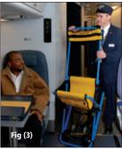
Pivot seat open, use foot to extend two inner wheels, assist passenger into chair.
