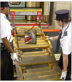
Figure 1-14 – Secure folding stairs to car body
