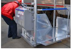
Figure 11-2 – Positioning Lift Next to Train
