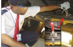
Figure 1-13 – Release folding stairs hold-down clamp
