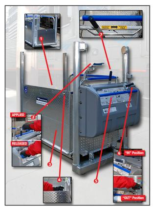
Figure 11-1 - Wheelchair Lift Components
