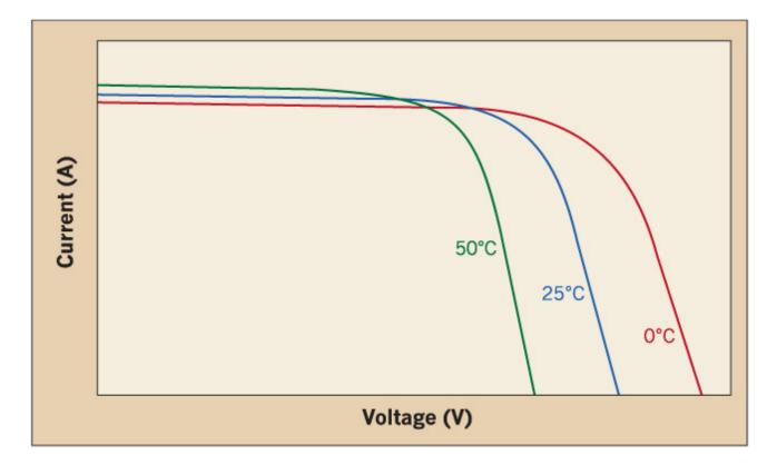
PV string - open circuit voltage changes with temperature!
