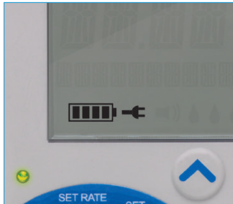
12. When the pump is powered by the AC/ mains a plug icon shows on the LCD and an LED light above the pump dial illuminates. These icons indicate the pump's integral battery is being recharged. During recharging the LCD battery icon will scroll. It may take up to 2 minutes for the green LED light to illuminate if the battery is depleted.
