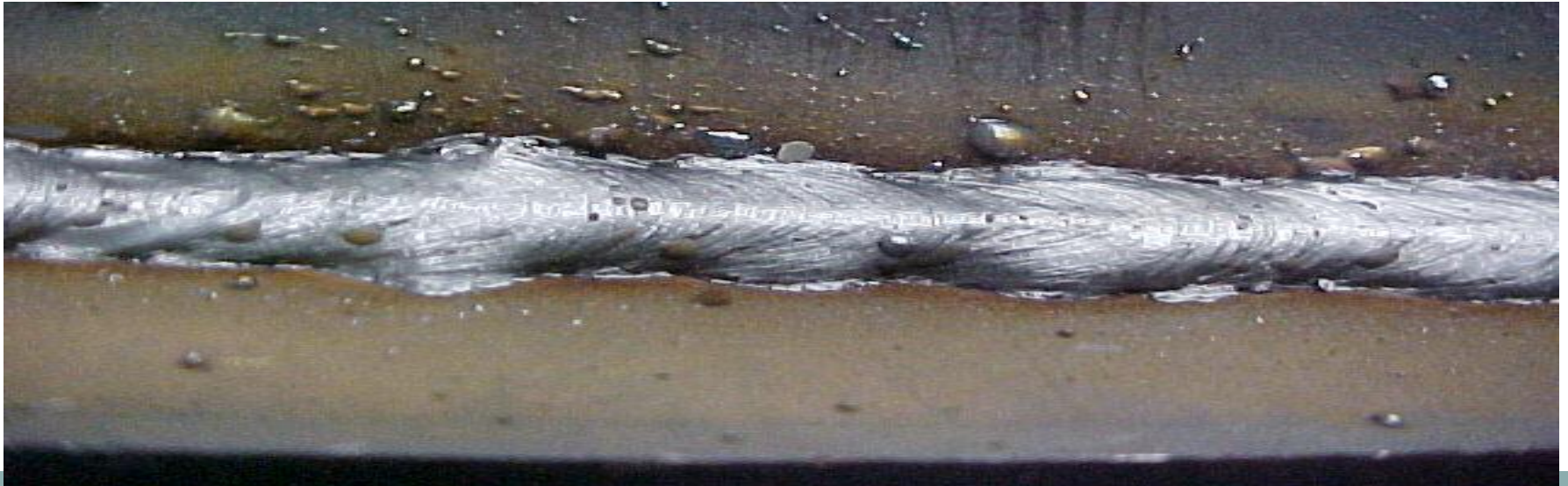
Overlap (Arrowed) and lack of fusion
