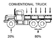
Tires, axles, and frame are designed to carry a load distributed as shown.
