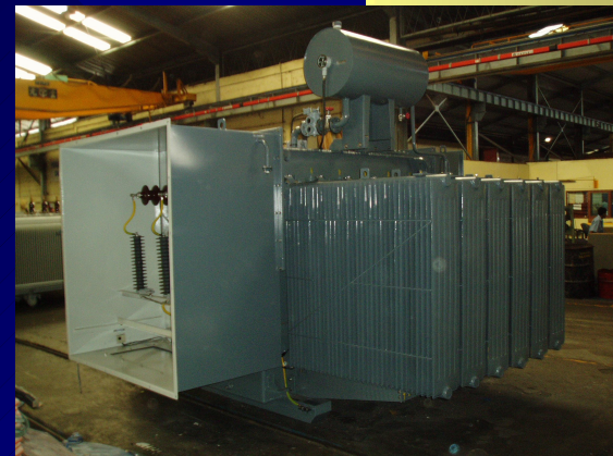
Conservator with rubber bag/diaphragm
