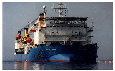
Barge (Shallow Water Cable Installer)
