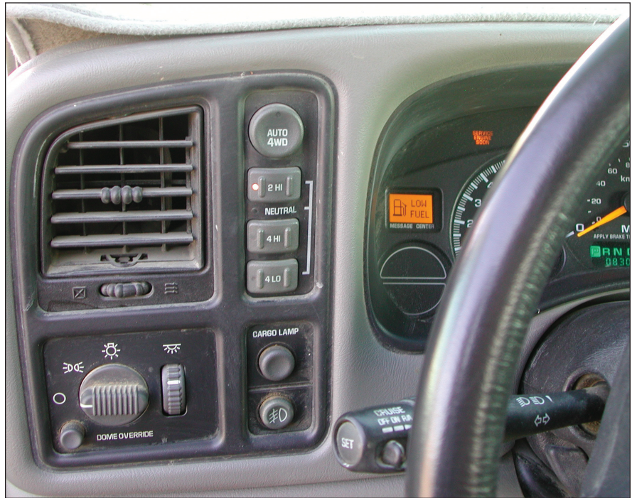
The dash buttons to the right of the air vent identify this system as an NVG 246 automatic two-speed, which means it has DTCs and scan tool capabilities.
