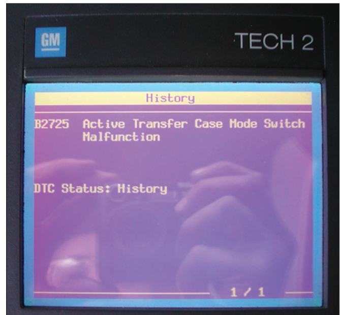
Left: ATC information can be found under the Powertrain menu on the Tech 2 scan tool. Other scan tools may allow access to these features as well. Right: A scan tool is also required to access DTCs. History and current DTCs are displayed on different menus (History menu shown here). DTCs will stay in memory for 100 key cycles.
