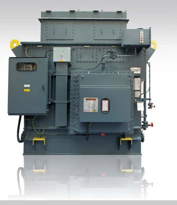
The AE series on-load tapchangers are built on the successful results of the design of the AT range. The AE uses many common parts from the AT including the complete drive mechanism. This range has a maximum of 17 tapping positions (16 steps) and is possible for linear regulation and 33 tapping positions (32 steps) for reverse or coarse/fine regulation.
