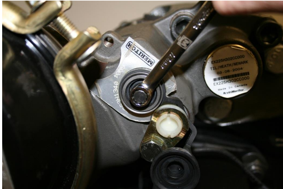
FIGURE 15 Meritor Brake Adjuster Setting
