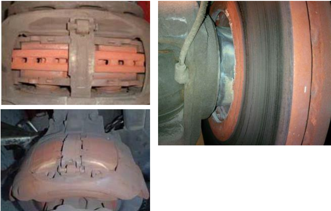
Bright-red coloration indicating brake overheating condition
