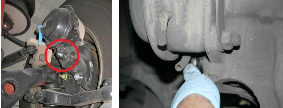
FIGURE 13 Brake Adjuster Inspection Locations
