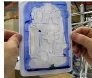
Seal integrity testing
