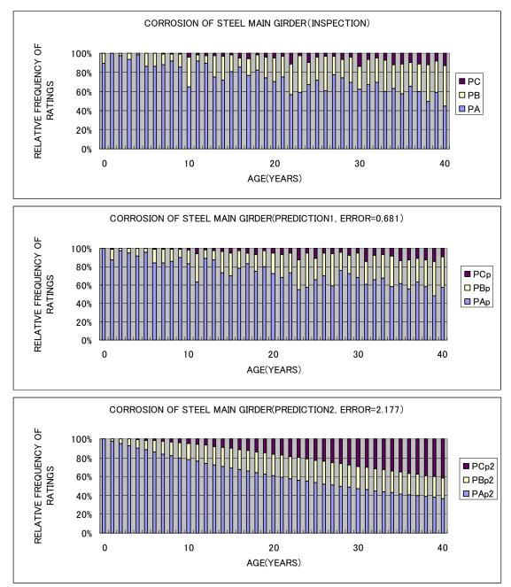
FIG. 2.1 DISTRIBUTION OF DAMAGE RATING FOR CORROSION OF STEEL MAIN GIRDERS (TOP: INSPECTION (SOURCE: MINISTRY OF LAND, INFRASTRUCTURE, TRANSPORT, AND TOURISM), MIDDLE: PREDICTION1, BOTTOM: PREDICTION2, RIGHT: TRANSITION PROBABILITY MATRIX OBTAINED FROM METHOD2)
