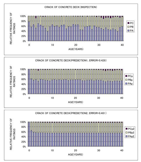
FIG. 1.3 DISTRIBUTION OF DAMAGE RATING FOR CRACK OF CONCRETE DECK (TOP: INSPECTION (SOURCE: MINISTRY OF LAND, INFRASTRUCTURE, TRANSPORT, AND TOURISM), MIDDLE: PREDICTION1, BOTTOM: PREDICTION2, RIGHT: TRANSITION PROBABILITY MATRIX OBTAINED FROM METHOD1)
