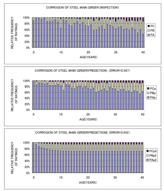
FIG. 1.1 DISTRIBUTION OF DAMAGE RATING FOR CORROSION OF STEEL MAIN GIRDERS (TOP: INSPECTION (SOURCE: MINISTRY OF LAND, INFRASTRUCTURE, TRANSPORT, AND TOURISM), MIDDLE: PREDICTION1, BOTTOM: PREDICTION2, RIGHT: TRANSITION PROBABILITY MATRIX OBTAINED FROM METHOD1)
