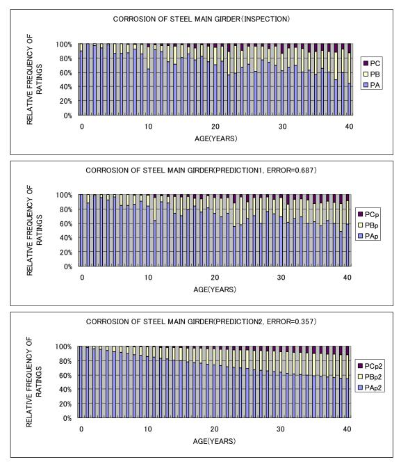
FIG. 2.2 DISTRIBUTION OF DAMAGE RATING FOR CORROSION OF STEEL MAIN GIRDERS (TOP: INSPECTION (SOURCE: MINISTRY OF LAND, INFRASTRUCTURE, TRANSPORT, AND TOURISM), MIDDLE: PREDICTION1, BOTTOM: PREDICTION2, RIGHT: TRANSITION PROBABILITY MATRIX OBTAINED FROM METHOD3)
