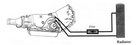
Picture shows a typical filter installation where the top line is the return line. If the "rear" or "bottom" line is the return line, the filter would be installed into it with the direction of flow toward the transmission. Refer to chart below for return line identification.
