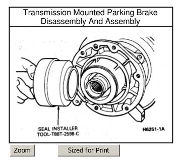
25. Coat the outer shell of a new inner oil seal with sealer and install it in the bore of the case until it seats inside the bore. The sealing lip of the seal must face inward.
