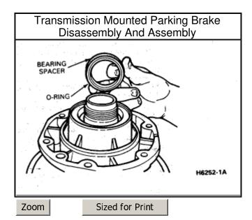
26. Install a new O-ring in the notch of the bearing spacer and install both parts onto the mainshaft until the space butts against the shoulder of the shaft.
