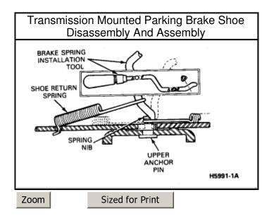
3. With the upper ends of the shoes against the upper anchor pin, install two new shoe return springs. Install the short hooked end of each spring into the upper holes of the <a href="brake shoes">brake shoes</a> and hook the opposite end of each spring over the anchor pin nib, using a suitable spring installation tool. Be sure the open end of the spring hook faces toward the brake centerline.
