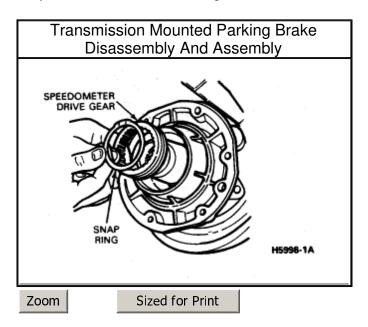
16. Install the speedometer drive gear onto the mainshaft. Install the snap ring into the groove locking the speedometer gear to the shaft.
