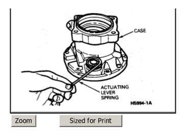
6. Install the actuating lever spring in the boss in the case.
