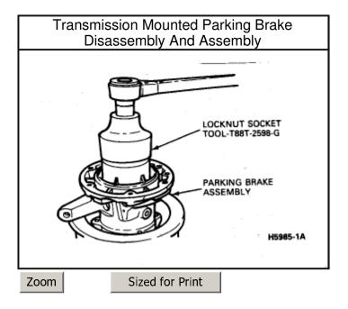
19. With the case assembly and mainshaft clamped firmly in the vise, screw the hex locknut onto the mainshaft. Tighten the nut to **288-292 Nm (212-216 ft-lb)** .
