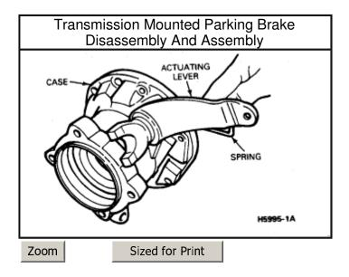
7. Apply a light coating of Ford Disc Brake Caliper Slide Grease D7AZ-19590-A, or equivalent to the ball of the actuating lever. Install the lever (ball end) into the hole in the boss of the case, through the coiled end of the spring.
