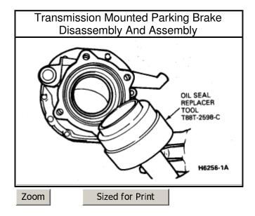
5. Apply a light coating of sealer to the outer edge of the outer oil seal. Position the oil seal in the bore of the case with the sealing lip facing inward. Press the seal into the bore of the case using tool T88T-2598-C, or equivalent. Press the seal in flush with the bore surface.
