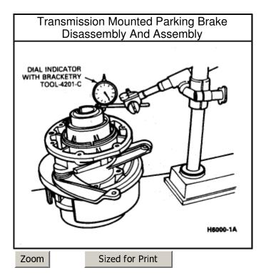
20. Mount a dial indicator between the mainshaft and the case to check end play. Use dial indicator with bracketry Tool-4201-C or equivalent.
