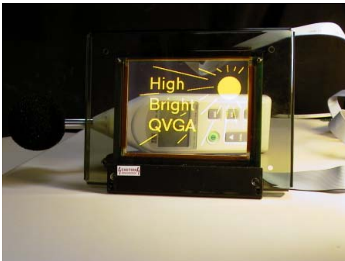
Figure 9 - A quarter-VGA transparent electroluminescent display
