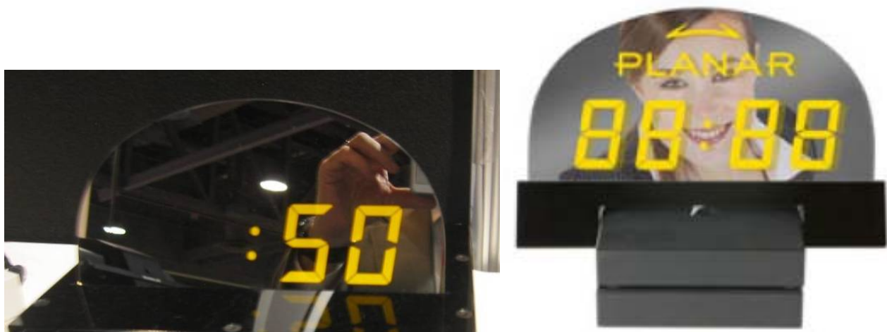
Figure 13 - Transparent TFEL display with a front surface mirror provides new options and effects
