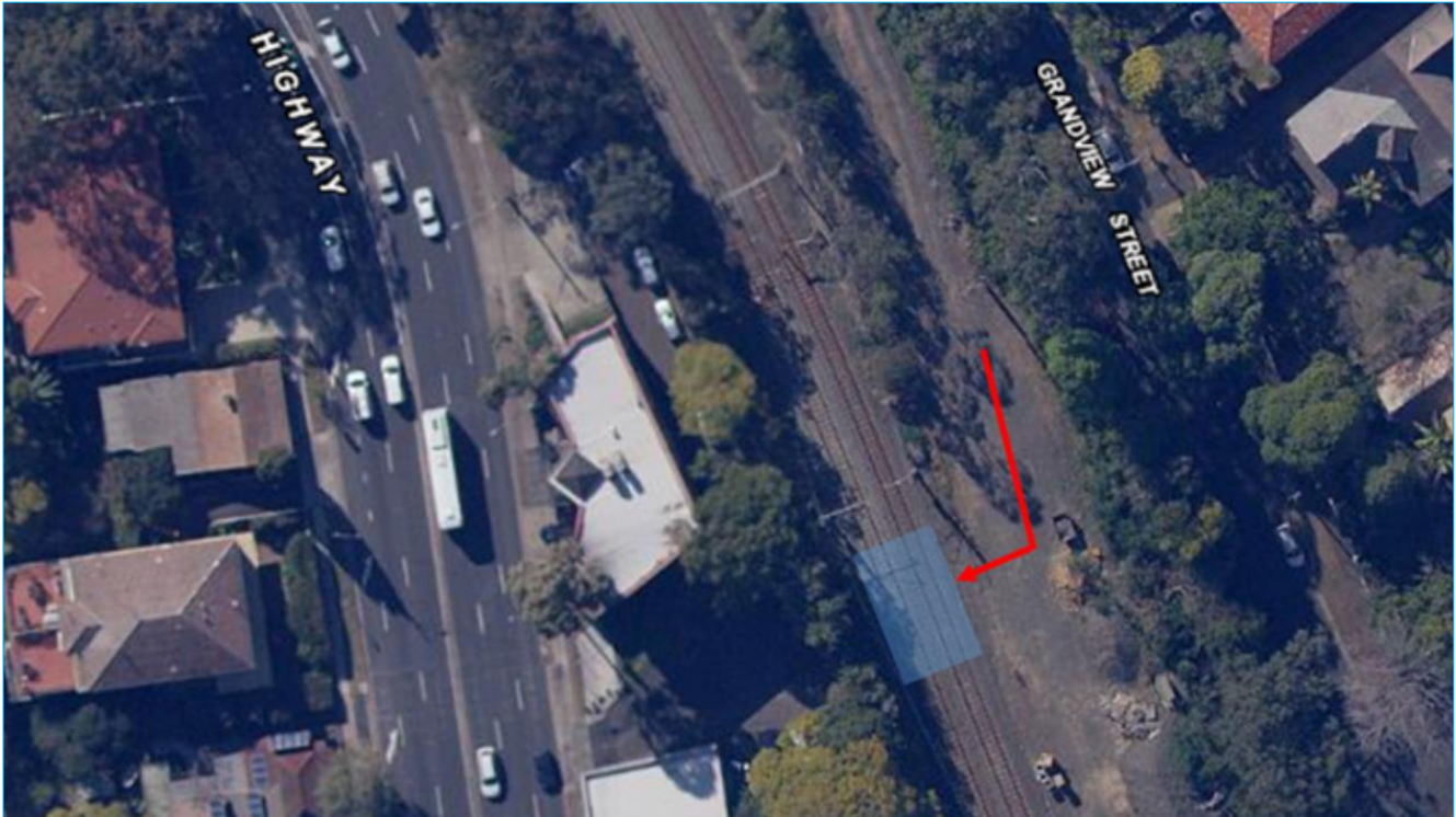
Figure 31: Hi-Rail Vehicle Access to Rail Tracks via Grandview Street, Pymble
