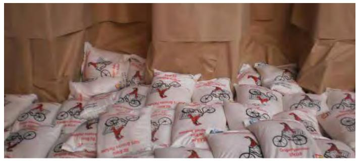
**Figure 3.10 |** The transverse bulkhead in the background is covered with kraft paper. Note how bags are placed tightly into the bulk head. No space is wasted.
