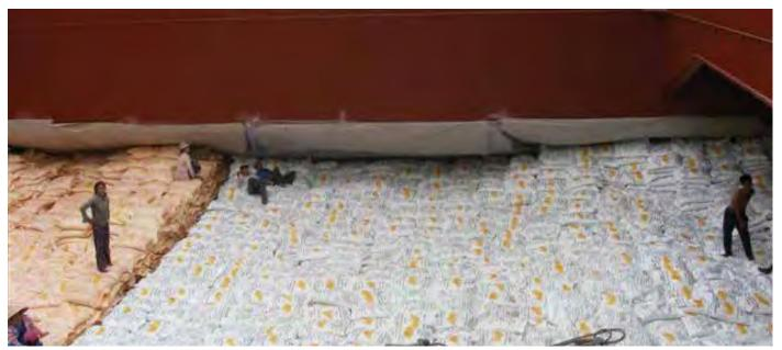
Figure 3.11 | Note the kraft paper covered by plastic/polyethylene sheeting on the top side of the top sloping tanks.
