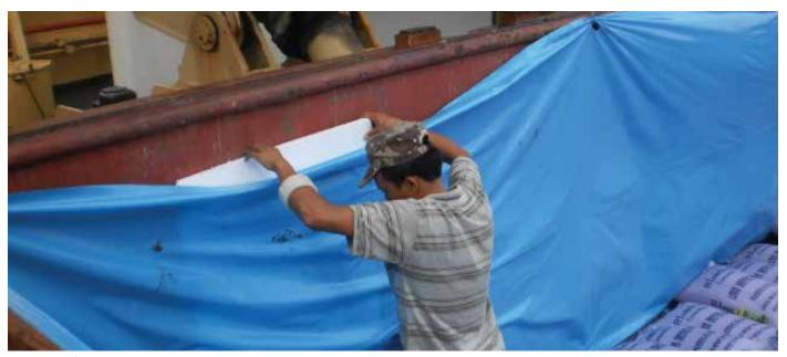
Figure 3.13 | Stevedore inserting Styrofoam sheet between hatch coaming and plastic sheeting.
