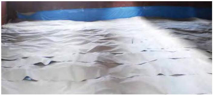
Figure 3.16 | Cargo is loaded to the foot of the hatch coaming and covered with kraft paper.
