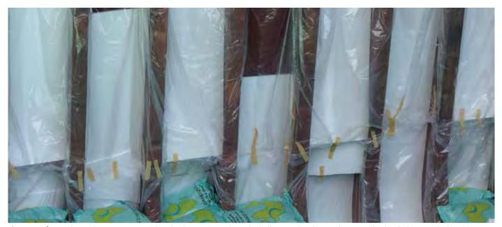
**Figure 3.8 l** Styrofoam sheets are covered with plastic along the sideshell. Note that bags of rice can be loaded to touch the plastic sheeting so moisture from ship sweat cannot penetrate.
