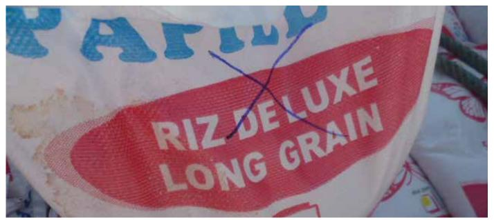
Figure 1.7 | Water damage on a rice bag resulting from the accumulation of condensation.
