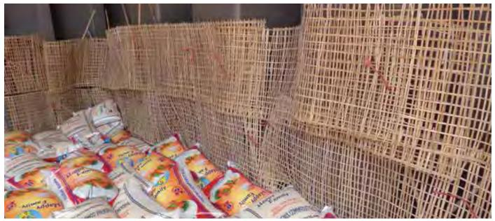
Figure 3.3 | Bamboo mat dunnage placed along a corrugated transverse bulkhead.
