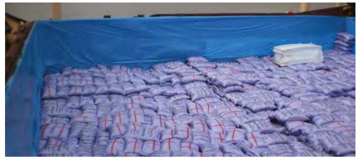
**Figure 3.14 I** Cargo is stacked to the foot of the hatch coaming. Note the stack of Styrofoam sheets used for insertion between the hatch coaming and plastic sheeting.
