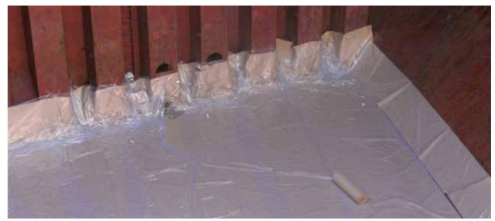
**Figure 3.5 I** The cargo hold top tank, base of the transverse corrugated bulkhead and base of the hopper tank top have been lined with kraft paper overlaid with clear plastic sheeting.
