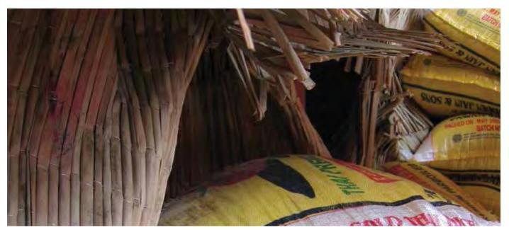
**Figure 3.4 I** Bamboo mat dunnage placed along the ship sideshell has been stained by ship sweat. The bag adjacent to the dunnage has been stained as a result of the migration of water though the bamboo matting.
