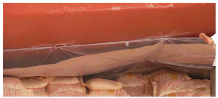
Figure 3.12 | Cargo loaded to the foot of the hatch coamings. Note the kraft paper covered by plastic sheeting on the top sloping tanks.
