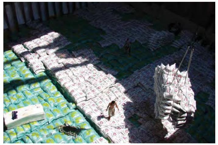
**Figure 4.1** I Stevedores loading and stacking bags with ventilation channels between stows. In the background, note the Styrofoam covered by plastic along the sideshells.
