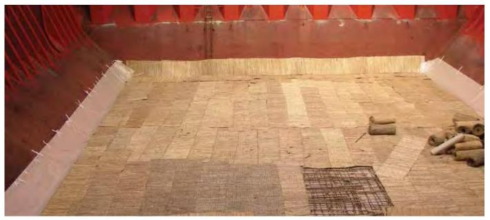
**Figure 3.1** An example of a cargo hold being prepared for the transport of bagged rice. Note the vessel's tank top being lined with cross bamboo sticks and bamboo matting lay atop. Kraft paper is used for lining the hopper tanks.
