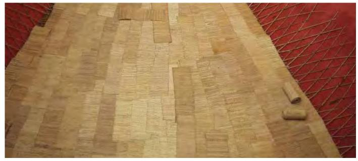
**Figure 3.2** | A cargo hold being prepared to transport a consignment of bagged rice. Note the vessel's tank top being lined with cross bamboo sticks and bamboo matting lay atop.
