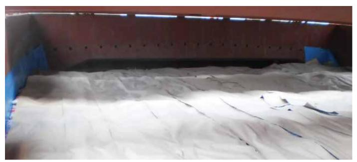
**Figure 3.15 I** Cargo is loaded to the foot of the hatch coaming and covered with kraft paper. Also note the plastic sheeting protruding out of the sloping wing plates and taped to the hatch coamings.
