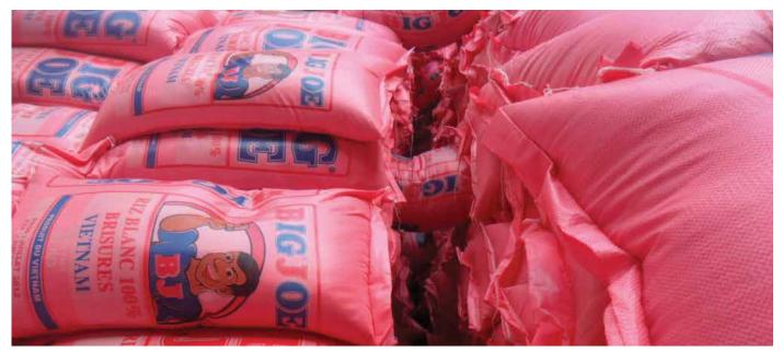
**Figure 4.7 I** Ventilation channel between stacks of bagged rice. Note that every 5 or 6 tiers, that a rice bag is set across stacks interlocking the tiers. This is done so to stabilize the stacks of cargo preventing collapse and shifting of stacks.
