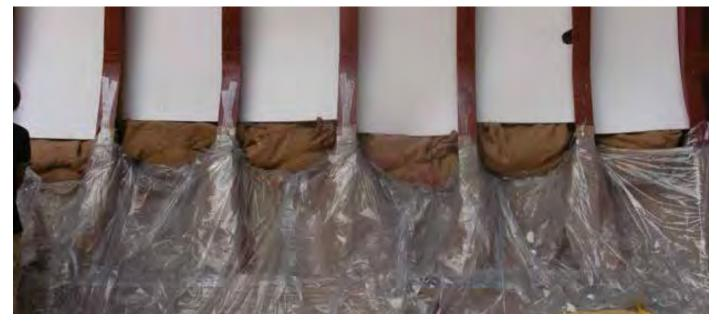
Figure 3.18 | Saw dust in burlap bags is inserted at transition point between sideshell and the top of the hopper tank.
