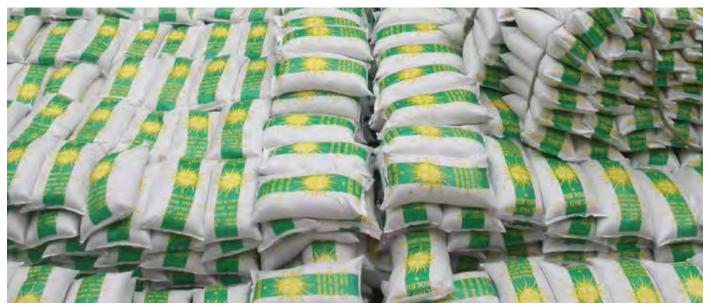
**Figure 4.8 I** Note in the center foreground of the picture the bags laid across the ventilation channel running left to right interlocking the tiers. This is done so to stabilize the stacks of cargo preventing collapse and shifting of stacks.
