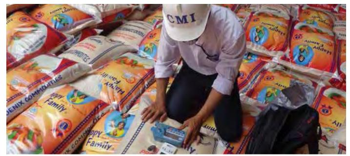
Figure 4.5 | A cargo surveyor taking moisture content measurements directly from a stowed bag of rice in the cargo hold.
