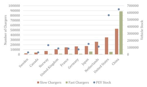
Fig. 2. Number of public slow (level 1–2) and DC fast chargers, and number of PEVs registered in the top 10 PEV markets. The number of charging stations differs between regions, and is related to the number of PEVs, travel patterns, housing type and other factors associated with local market conditions (International Energy Agency, 2017).
