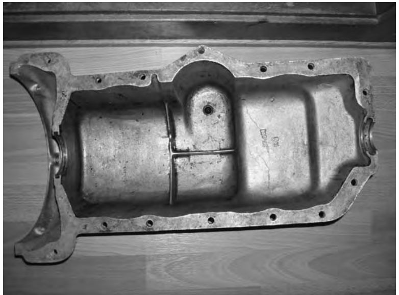
The aluminium sump on Harley Gausen's early Model "Y". Note the oil drain hole under the oil pump and the extra bolt hole alongside the oil pump space and the round front packing seal recess on the aluminium sump, dating the engine post late summer/autumn 1938.
