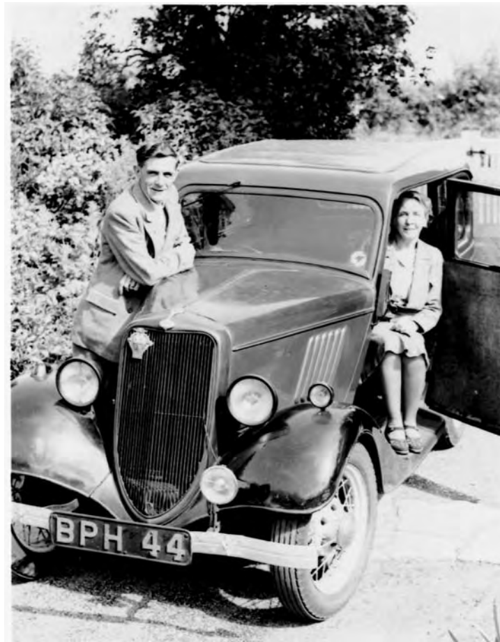
Mr and Mrs White in their 1934 Tudor Model "Y" in 1950. Note the early piano hinged bonnet, the almost essential 'smog' light and the modified nearside side lamp - I wonder why that was?
