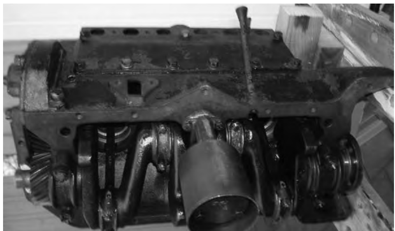
The extra bolt hole clearly visible on the triangular oil pump surround on the crank case. Note also the dip stick tube, which was not fitted before August 1938."
