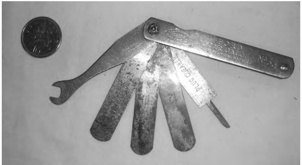
This larger set is inscribed, 'FORD CAR GAUGE' No. 35 CONSULT THE BOOKLET'. It was manufactured by Moors & Wright of Sheffield (Patent no. 792592) and consists of a small spanner (not large enough for the distributor nuts), gauges marked 'SPARK PLUG 25', 10 and 12 and a pointed scraper marked 'PLUG CLEANER'
