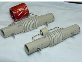
Photo A: Home-built Trap Capacitors
