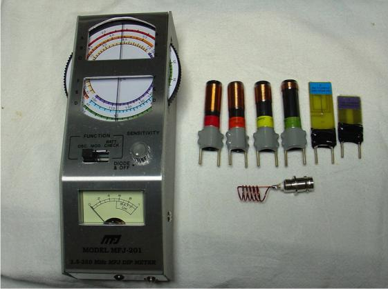
Photo D: The MFJ-201 Grid-Dip Oscillator
