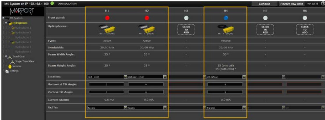
Figure 7: Hydrophone configuration for Slant Range sensors
