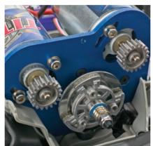
A Revo style slipper clutch protects the transmission from any sudden shock and it's fully adjustable.
