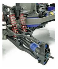
The driveshafts and hubs are also borrowed from the Revo. Dual shocks control the suspension arms on each corner of the truck.
