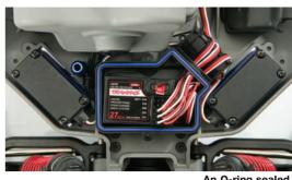
An O-ring sealed radio box keeps water and debris away from the receiver.
