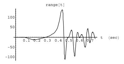
Fig. 13. The behavior when the sling is very short (0.5 ft in the example).
