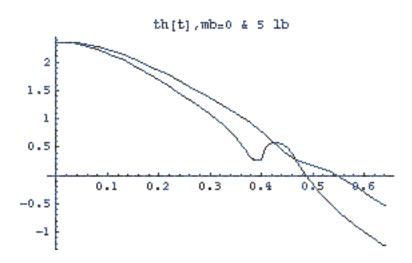
Fig. 8. A comparison of the (t) solutions for trebuchets with mass zero amd mb=5 compared. The mb=0 case has a minimum at time 0.4.
