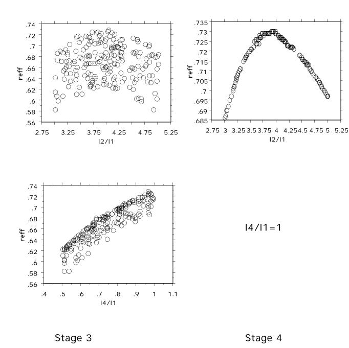
Fig. 21. Stages 3 and 4 of the Monte Carlo exploration. In both of these simulations psiz is constrained to  $45^{\circ}$  and the sling length/long arm ratio is unity.
