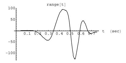
Fig. 12. The behavior of the trebuchet for a shortened sling.
