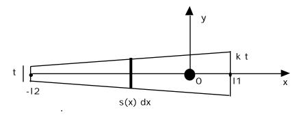
Fig. 22. The linear non-uniform beam with mass per unit length s(x), thickness t at the sling end and k t at the CW end.
