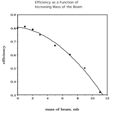
Fig. 9. The effect of the mass of the beam on the efficiency of the trebuchet.
