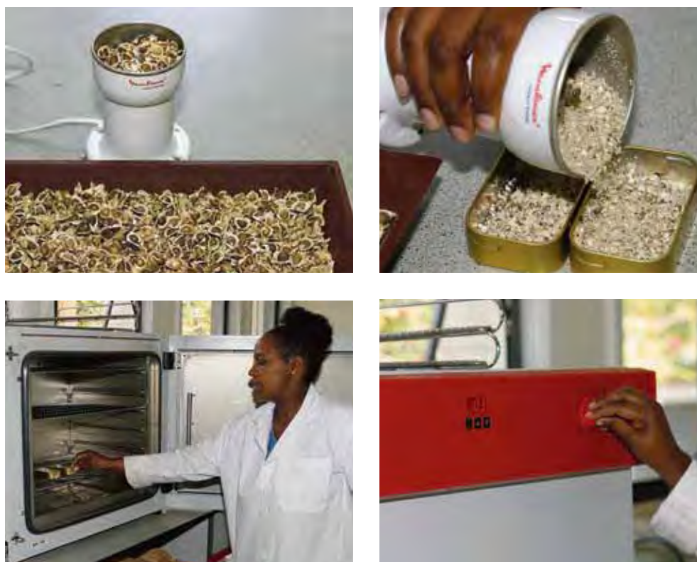
Figure 12.4 Measuring moisture content using a low constant-temperature oven
