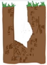
Closed Lip Failure
