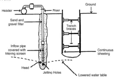
Well-points are pipes with a point at the lower end and a screen or filter over perforations along 3 or 4 feet of the lower ends of the pipes. There are two types of well-points:
