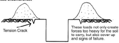
Existing site features such as buildings, curbs, trees, utility poles and other structures adjoining the excavation area may be considered as types of surface encumbrances. These extra loads can place more stress on the sides of an excavation than the walls can safely carry. Shoring, bracing, underpinning or some combination of safety measures should be provided, as necessary, to protect workers and to prevent movement of the soil beneath the adjacent load.
