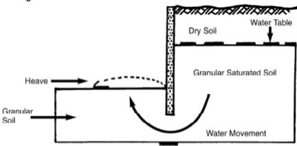
Wet conditions at the bottom of a trench may present another problem. If the bottom of the trench begins to puff and bubble and the earth rises, a quicksand condition is occurring. This is also a signal that a failure may occur.
