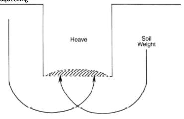
Boiling is evidenced by an upward water flow into the bottom of the cut. A high water table is one of the causes of boiling. Boiling produces a "quick" condition in the bottom of the cut and can occur even when shoring or trench boxes are used. See Figure 7.
