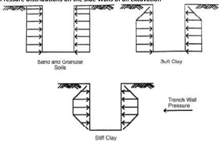
As a general rule of thumb, the center of pressure will be at a lower depth when cohesion is poor (as in fresh fill dirt, water-bearing sand or loose ground). Where cohesion is high, the center of pressure will be higher (as in good compact soil). The location of the center of pressure can change after a cut is made unless support is provided to prevent earth movement.
