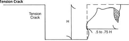
Sliding or sluffing may occur as a result of tension cracks, as illustrated in Figure 3.
