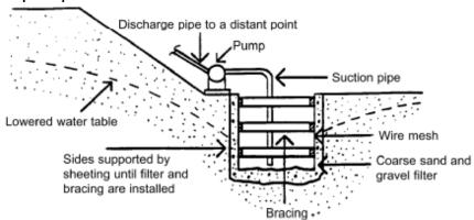
Sump pumping, as contrasted with well-pointing, has several advantages. Sump pumps:
