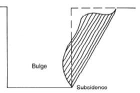
**Heaving or Squeezing**. Bottom heaving or squeezing is caused by the downward pressure created by the weight of adjoining soil. This pressure causes a bulge in the bottom of the cut, as illustrated in Figure 6. Heaving and squeezing can occur even when shoring or shielding has been properly installed.
