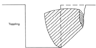
Subsidence and Bulging. An unsupported excavation can create an unbalanced stress in the soil, which, in turn, causes subsidence at the surface and bulging of the vertical face of the trench. If uncorrected, this condition can cause face failure and entrapment of workers in the trench. See Figure 5.
