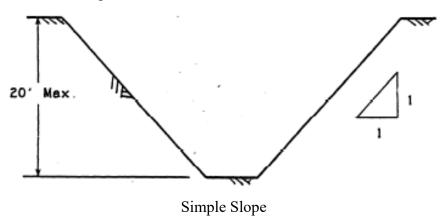
2 All benched excavations 20 feet or less in depth shall have a maximum allowable slope of 1:1 and maximum bench dimensions as follows:
