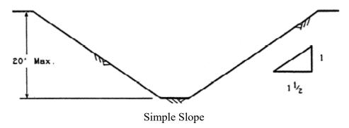
2. All excavations 20 feet or less in depth which have vertically sided lower portions shall be shielded or supported to a height at least 18 inches above the top of the vertical side. All such excavations shall have a maximum allowable slope of 1½:1.
