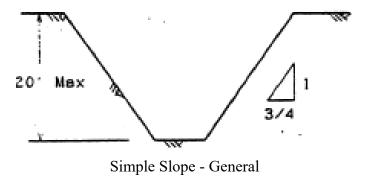
Exception: Simple slope excavations which are open 24 hours or less (short term) and which are 12 feet or less in depth shall have a maximum allowable slope of 1/2:1.
