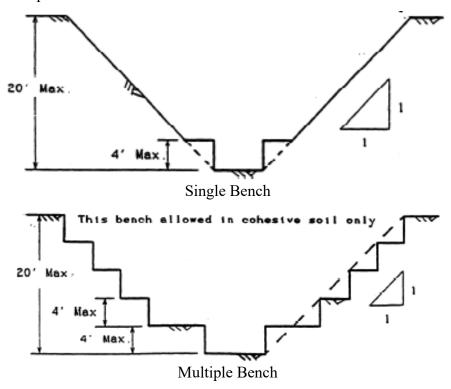
3. All excavations 20 feet or less in depth which have vertically sided lower portions shall be shielded or supported to a height at least 18 inches above the top of the vertical side. All such excavations shall have a maximum allowable slope of 1:1.
