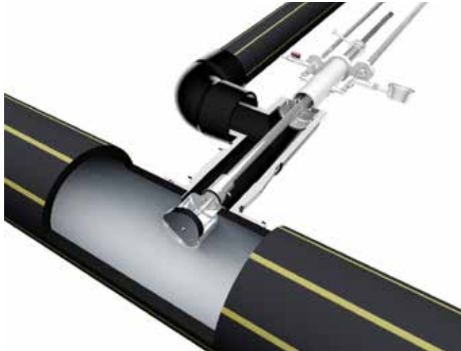
Figure 4 – Cutter Tapping PE Main Under Pressure
