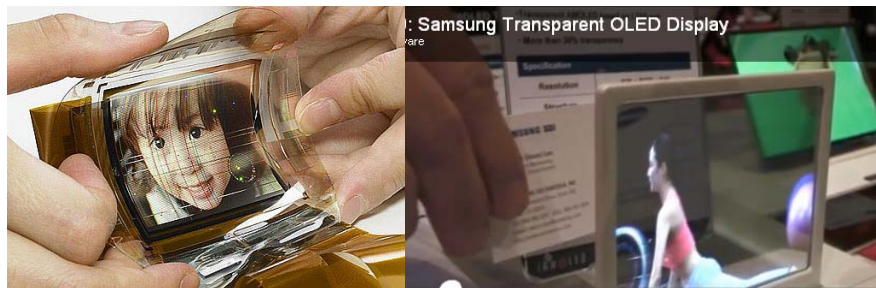
Figure 7a - OLED flexible displays (Pink Tentacle, 2011); 7b - Samsung transparent OLED display (CES, 2009)
