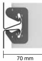
System depth with SE modular click rail
