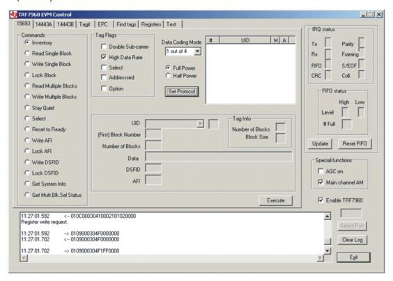
First Command: Register Write 01 0C 00 03 04 10 00 21 01 02 00 00 (all bytes are continuous; spaces are added for clarity)
