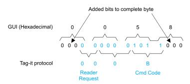
Figure 3-10. Quiet Request Packet Structure
