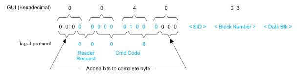
Figure 3-8. Lock Block Request Packet Structure
