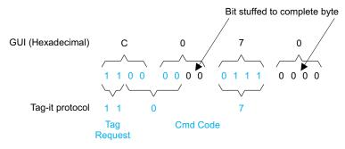
Figure 3-7. Put Block Lock Response Packet Structure
