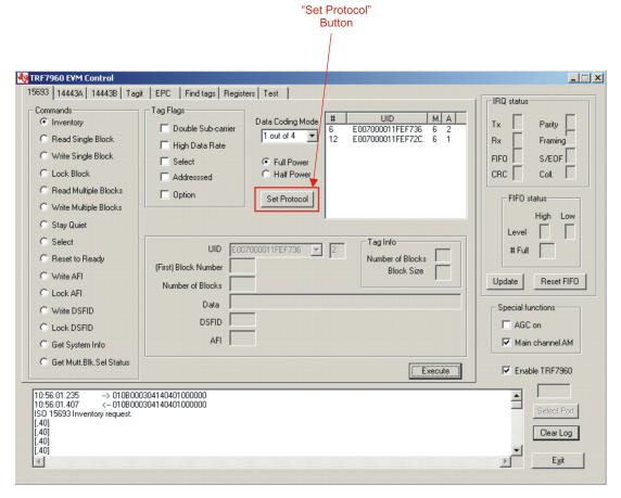
When the *Set Protocol* button is pressed, the software sets the parameters for the corresponding standard. These settings can also be modified through the *Registers* tab in the GUI.
