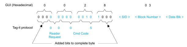
Figure 3-4. Put Block Request Packet Structure
