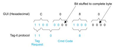
Figure 3-9. Lock Block Response Packet Structure
