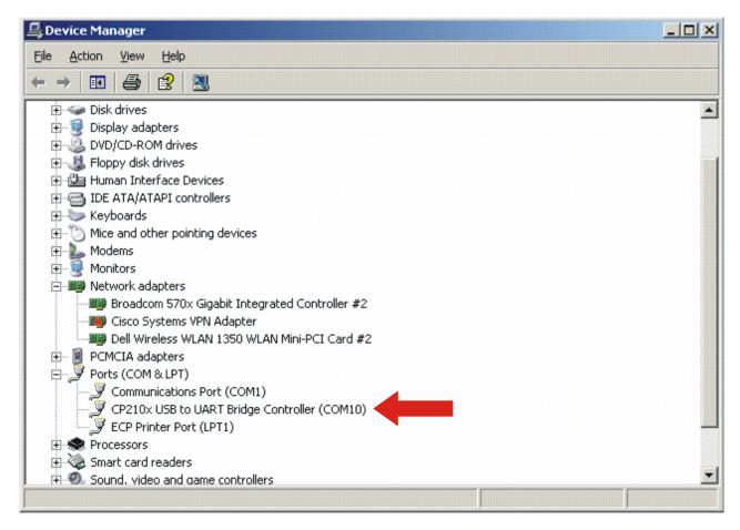
If the driver installation was successful and the EVM is plugged in, CP210x USB to UART Bridge Controller should appear in the list of ports, followed by a port number (in this example, COM10). The actual port number may be different.
