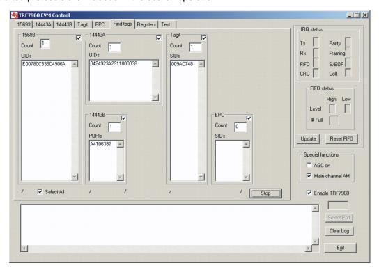
Once the *Run* button is clicked, the window shows all tags found within its reception area, regardless of protocol, if the *Select All* option is checked. Otherwise, it only finds tags of the protocols that are checked. This command runs until the *Stop* button is clicked (shared location with the *Run* button). An indicator for each of the supported standards is active when the particular protocol is running. This clockwise rotating cursor can be found located left of the *Run* button.
