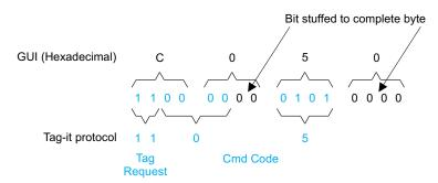
Figure 3-5. Put Block Response Packet Structure
