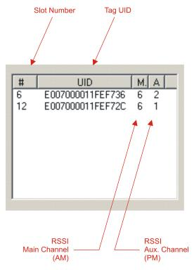
In the preceding example, one can see that the tags in slots #6 and #12 have a main-channel RSSI value of 6, with auxiliary-channel RSSI values of 2 and 1, respectively.
