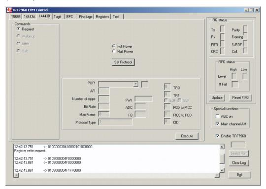
First Command: Register Write 01 0C 00 03 04 10 00 21 01 0C 00 00 (all bytes are continuous; spaces are added for clarity)
