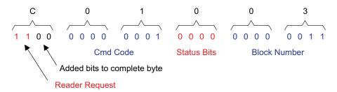
Figure 3-2. Get Block Response Packet Structure (Part 1)
