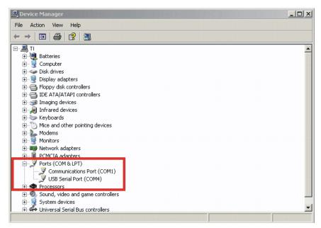
If the driver installation was successful and the EVM is plugged in, *USB Serial Port* should appear in the list of ports, followed by a port number (in this example, COM4). The actual port number may be different. Make note of the COM port number and enter it in the *Select Port* window of the GUI. Then select the *Select Port* on GUI (do not press the *Enter* key). Note: If the *Enter* key is pressed, the program ends and the GUI closes.
