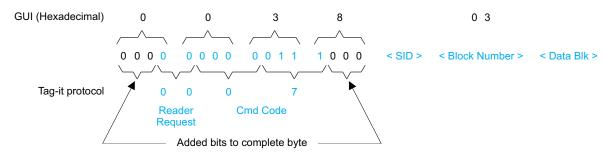
Figure 3-6. Put Block Lock Request Packet Structure
