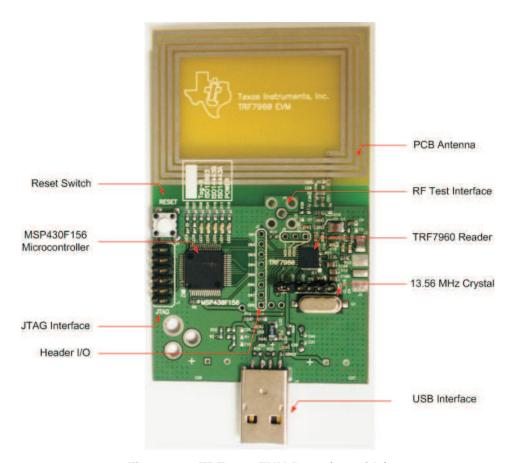
Figure 2-1. TRF7960 EVM Rev - (top side)
