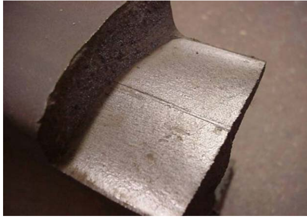
Figure 22: Horizontal Split Head Originating from Internal Seam
