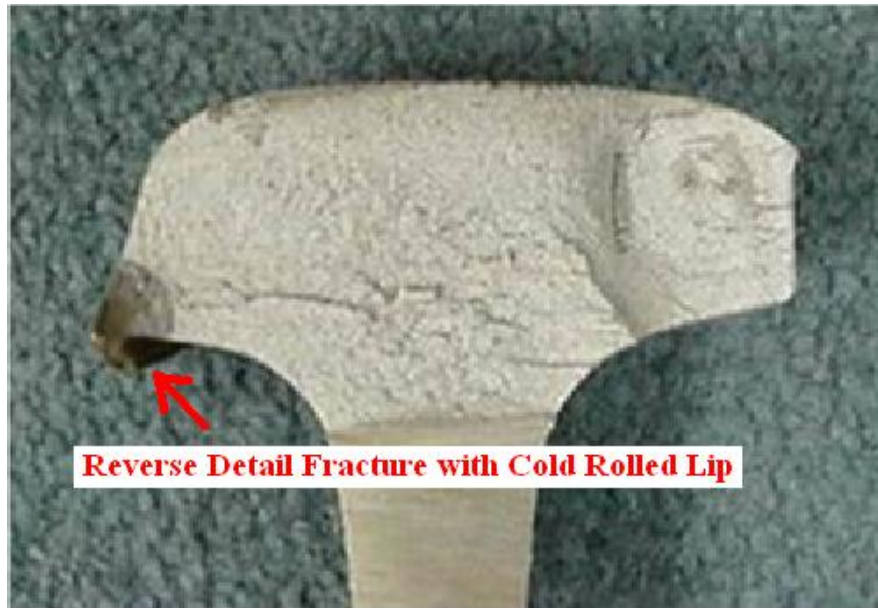
Figure 18: Reverse Detail Fracture
