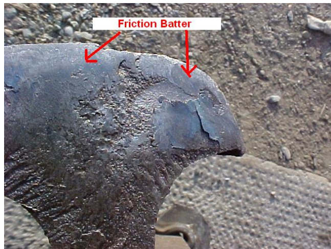
Figure 12: Friction Batter from Fracture Face Contact
