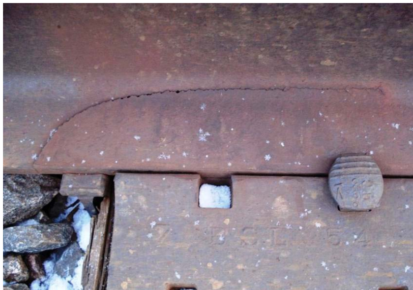
Figure 34: Half-Moon-Shaped Broken Base
