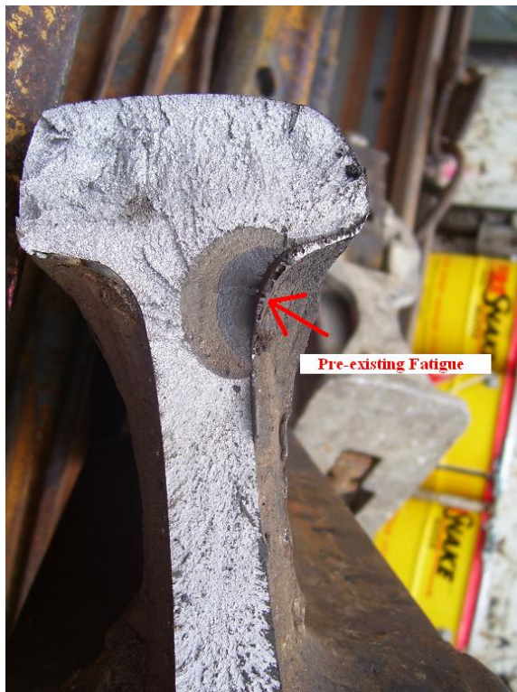
Figure 10: Weld Failure Showing Preexisting Fatigue and Second Stage Rupture
