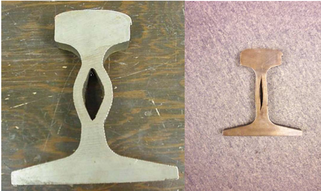
Figure 32: Piped Rail Showing Significant Rail Collapse
