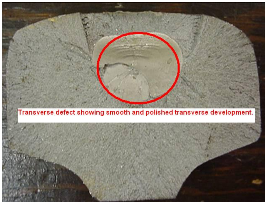
Figure 3: Transverse Fissure Showing Normal Growth Pattern.
