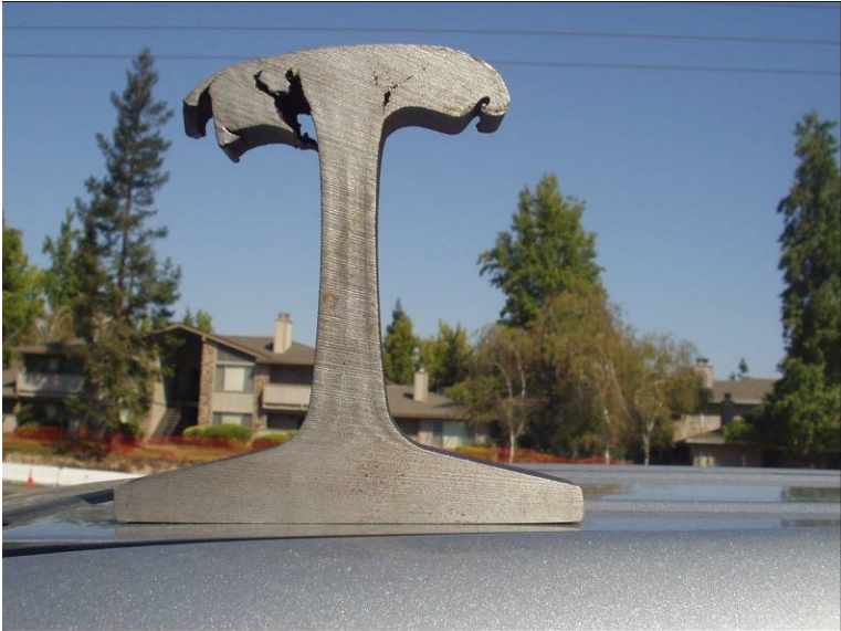
Figure 26: Vertical Split Head (Shear Break)
