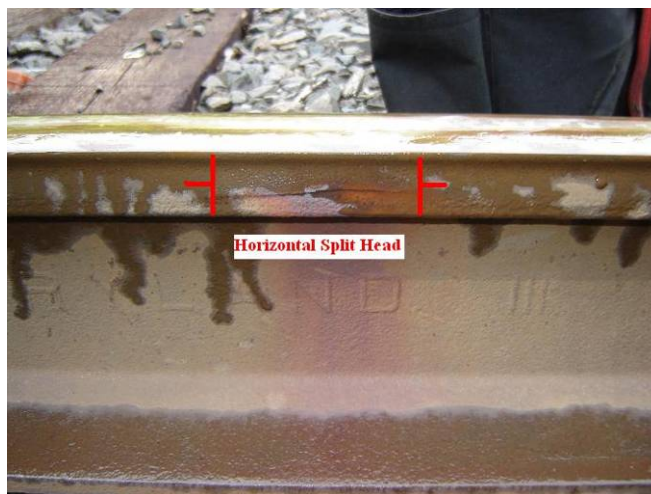
Figure 23: Side View of Horizontal Split Head
