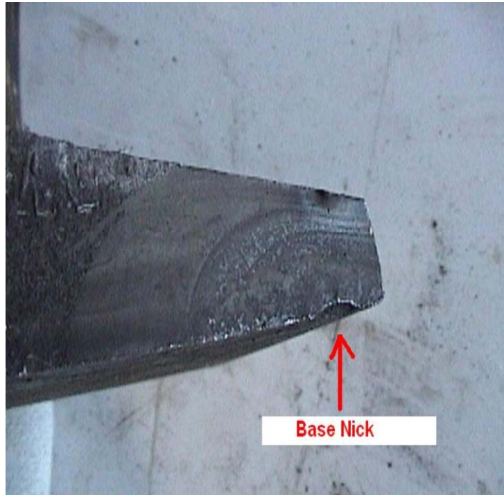
Figure 35: Base Fracture Showing Nick with Transverse Development
