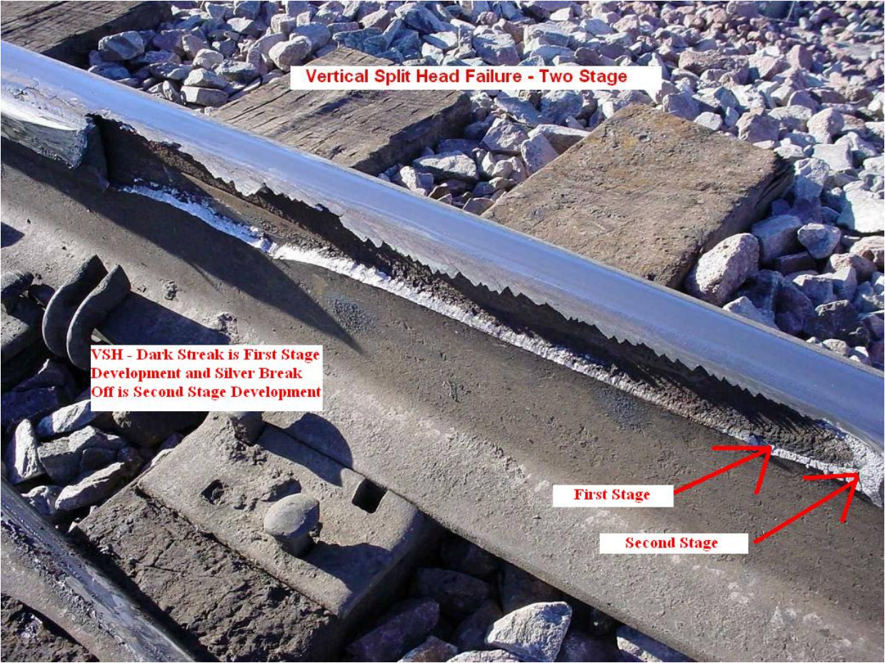
Figure 8: Vertical Split Head Showing Two-Stage Development
