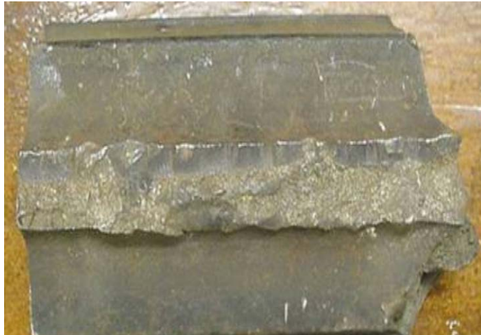
Figure 28: Head and Web Separation Showing Progression into Web
