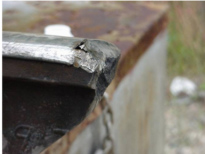
Figure 11: Impact Batter from Rolling Stock Wheels
