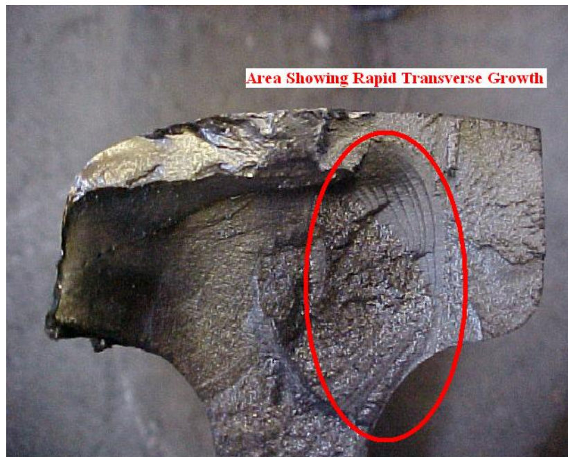
Figure 5: Compound Fissure Showing Segments of Rapid Growth Rings.
