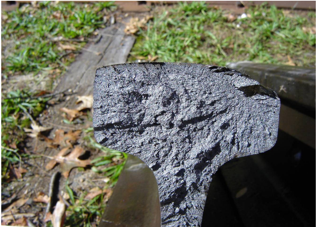
Figure 21: Rail Failure Fracture Face Showing No Transverse Defect
