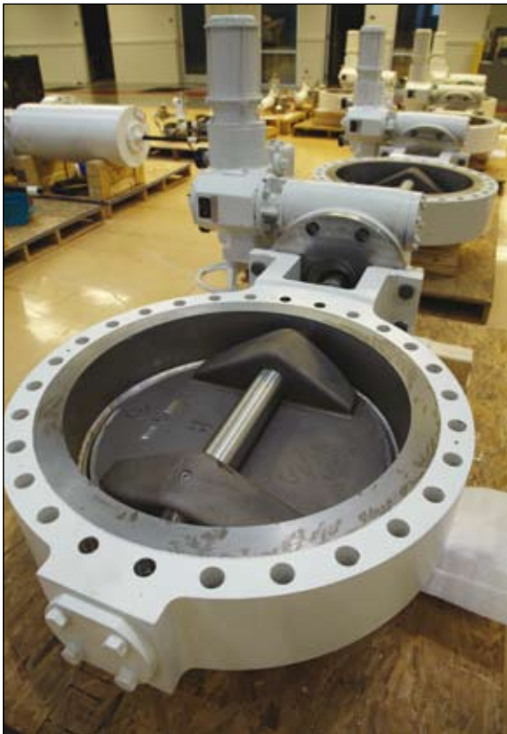
Motor operated valves in Ipswich, MA
