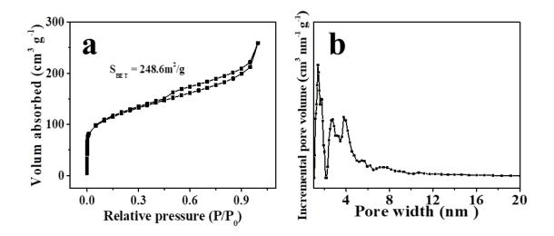
**Figure S4.** BET characterization of NiPG. (a) Nitrogen adsorption-desorption isotherm and (b) corresponding pore size distribution curve of NiPG.
