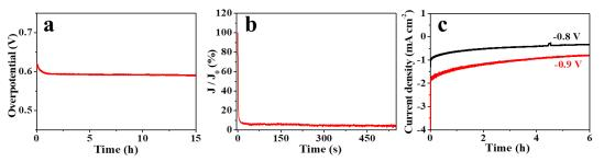
**Figure S11.** Electrocatalytic durability on NiPG in neutral solution. (a) OER and (b) ORR in 3 M KHCO<sub>3</sub> including 1.5 M KCl solution, and (c) CDRR in 0.1 M KHCO<sub>3</sub> solution, respectively.
