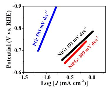
**Figure S9.** Tafel slope of CDRR on NiPG, NiG and PG. Electrolyte: 0.1 M KHCO<sub>3</sub> solution saturated with CO<sub>2</sub>.
