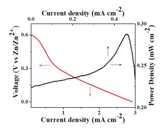
**Figure S13.** The Polarization and power density curves of rechargeable Zn-CO<sub>2</sub> batteries with NiPG as cathode.
