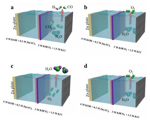
**Figure S12.** The scheme of aqueous rechargeable dual-model battery device. Zn  $CO_2$  battery mode of (a) discharge and (b) charge process. Zn  $O_2$  battery model of (c) discharge and (d) charge process.
