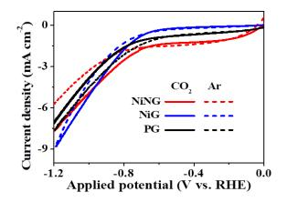
**Figure S8.** LSV scan of CDRR on NiPG, NiG and PG. Electrolyte: CO<sub>2</sub> saturated 0.1 M KHCO<sub>3</sub> solution.
