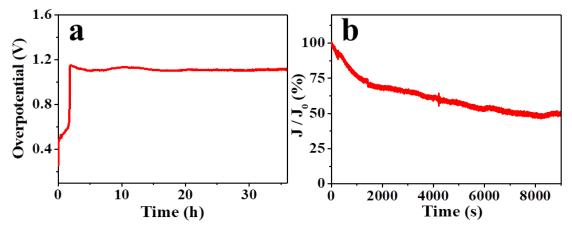
**Figure S10.** Electrocatalytic durability on NiPG in alkaline solution. (a) OER in 1 M KOH and (b) ORR in 0.1 M KOH solution.
