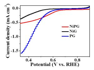
**Figure S7.** Neutral ORR performance on NiPG, NiG and PG. Electrolyte: 3 M KHCO<sub>3</sub> solution including 1.5 M KCl.
