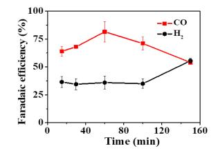
Figure S15. CO and  $H_2$  FEs of Zn-CO<sub>2</sub> batteries at discharge current of 0.5 mA.
