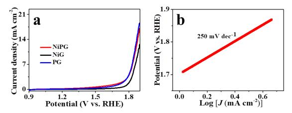
**Figure S5.** Neutral OER performance on NiPG, NiG and PG. (a) Neutral OER LSV curve and (b) Tafel slope of NiPG. Electrolyte: 3 M KHCO<sub>3</sub> solution including 1.5 M KCl.
