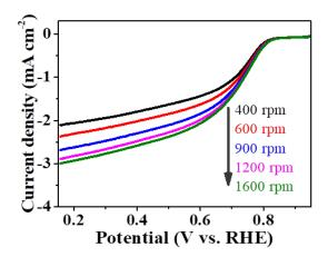
**Figure S6.** ORR LSV curves on NiPG at a series of rotating speeds. Electrolyte: 0.1 M KOH solution.
