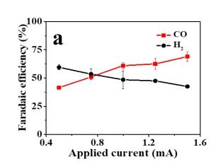
Figure S14. CO and  $H_2$  FEs of Zn-CO<sub>2</sub> batteries with error bar at a series of discharge currents.
