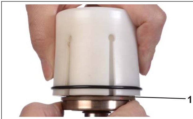
1. Seal installed in groove of piston 008834
