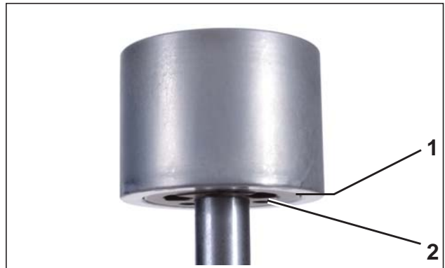
1. Bottom of the resizing fixture flush with the piston 008837 2. Piston
