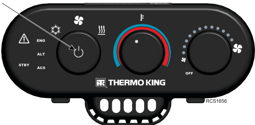
Figure 14. Press Mode Selector Knob to Turn System ON or OFF
